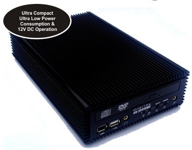
The CF50 from Digital Yacht measures just 160 x 55 x 250mm and runs directly from your 12V on board power system. It boasts a powerful Intel M processor, 256MB RAM and a 40GB hard drive with CDRW/DVD drive and full range of interfaces.
